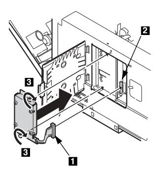
10. Close the access cover and slide it to secure it in the metal plate.
